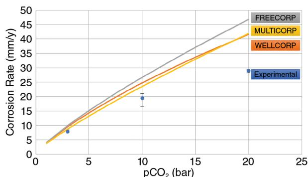
**FIGURE 1.** Comparison between corrosion models and experimental data, at 60°C, pH 5.0, 1 m/s, 1 wt% sodium chloride (NaCl), C1018 steel. Experimental data taken from Wang, et al.<sup>9</sup>
